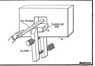
Fig. 17. Diagram Illustrating Method of Stoning out a Blanking Die
